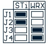
Depending on the country the vehicle was destined for the labelling of these jumpers (WRX and STi) may be incorrect. It may be necessary to try both options to determine which one is correct. If your vehicle is an STi and the ECU powers up with jumpers in the WRX position don't be alarmed.
